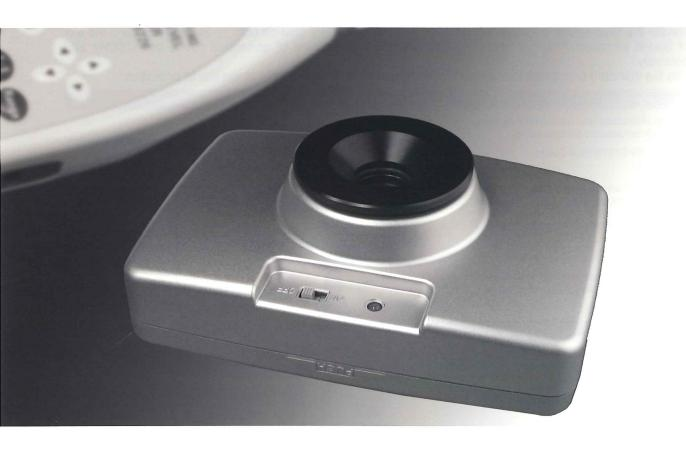
Compact, lightweight and easy to use You can use it easily in the calibration of precision sound level meter, all due to built-in microphone with temperature compensation.
